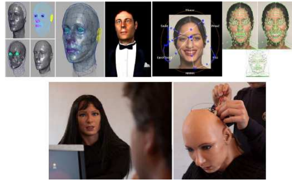
Fig. 2 The technology of high fidelity animated digital faces (Above) is used to evaluate an emotionally expressive physical robot (Below).
