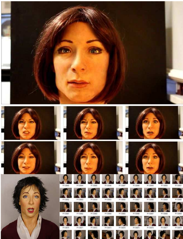
Fig. 3 Reference photos used to create 3D models of the FACE robot [12]. The two versions had different hair style and make up to simulate variations in appearance.
