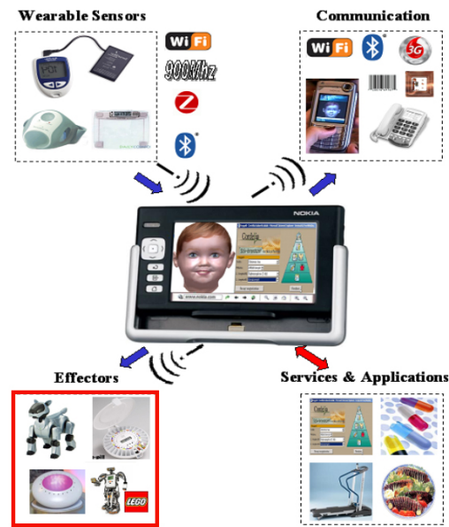
Figure 2. Overall modules of compliance monitoring for Ambient Assisted Living (AAL) and the role of effectors/robots in the home.
