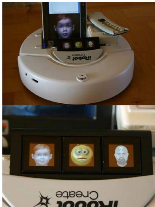
Figure 4. Ambinet Facial Interfaces or AFI's provide instant visual feedback and easy-to-understand display of compliance levels.
