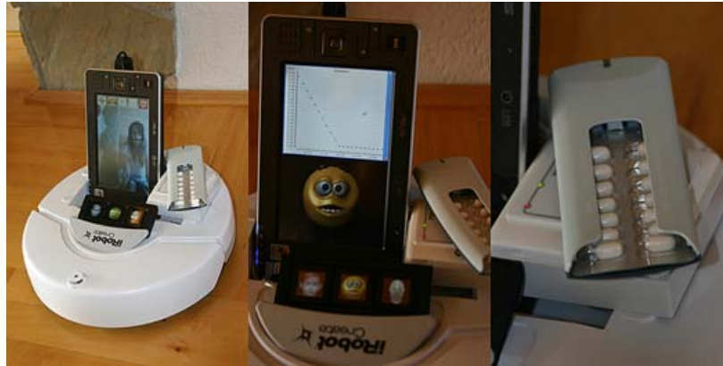
Figure 3. AAL Compliance robot in the home using face recognition, AFI's and an intelligent pilldispenser combined with RFID technology.
