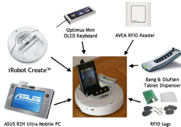
Figure 5. Hardware components integrated into our AAL robotic prototype solution.
