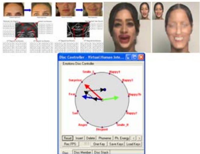
Fig. 14. Low level visual cues (edges, morphology, etc.) observed on a student's face are extracted and mapped onto an emotion disc as competing 'clues'.
