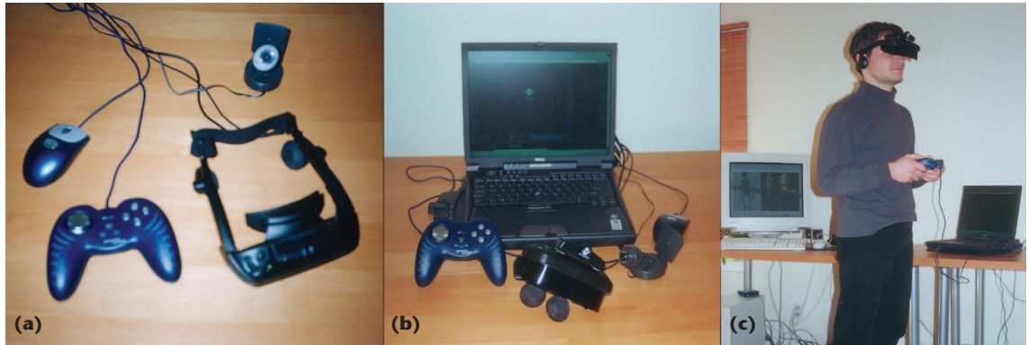
6 External virtual-reality devices that connect to the VHI system: (a) From left to right, magnetic motion tracker, joystick, head-mounted display, and video camera used for live input; (b) Complete portable system, and (c) user interacting with and experiencing a virtual environment.
